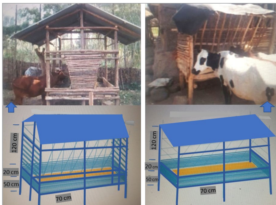
Figure 15. Layout and dimensions of two-sided (left) and one-sided (right) feeding troughs for cattle. Depending on the economic status of the farmers or cooperatives, the barn roof can be made from locally available materials such as grass mat or from manufactured plastic and corrugated iron sheets. The length, width, and height are determined by considering the average size of cattle of different breeds
