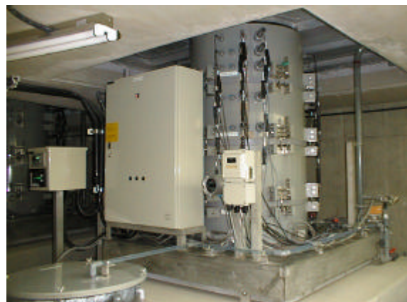
Fig.17. Lysimeter column segment and a large-sized electronic balance.
